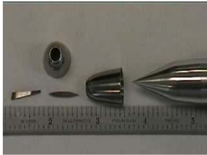
Figure 11. ABLE model parts: cowl nose cap, forebody, and struts.
